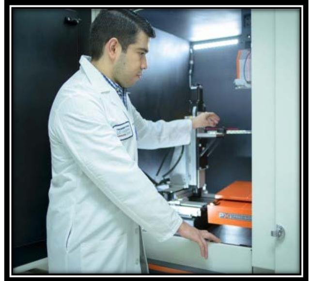
Dr. Jimenez inspecting a state-of-the-art biological irradiator that permits image-guided radiation therapy of small animals using built-in CT and bioluminescence imaging.
